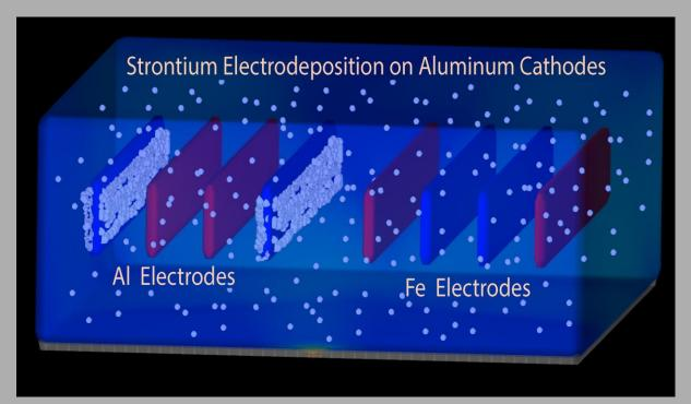
Selenium and strontium were electrochemically removed from the solution in a short operating time.
